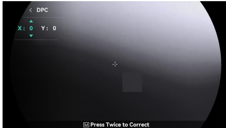
Figure 3-5 Correct Defective Pixel
